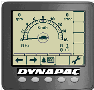
Fig. The display shows the selection in the middle (tortoise, drum spin, wheelspin or hare).
